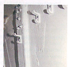
Timber is used to reinforce the bulkhead to chainplate attachment
