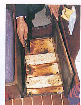
Check for corrosion of the steel keel fastenings. Hairline cracks in the reinforcement indicate stress
